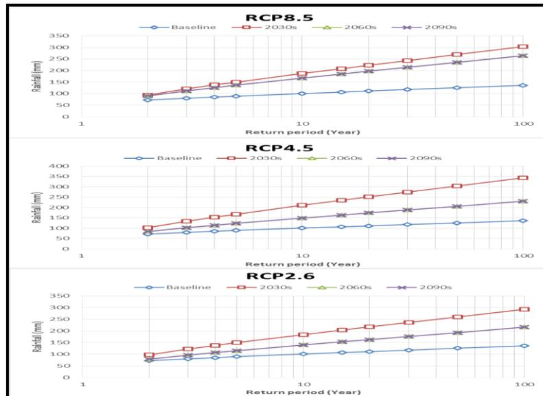
**Figure 12. Comparison of Gumbel estimated magnitudes of rainfall for studied return periods using AM series for baseline, 2030s, 2060s and 2090s under RCP 2.6, RCP 4.5 and RCP 8.5**
