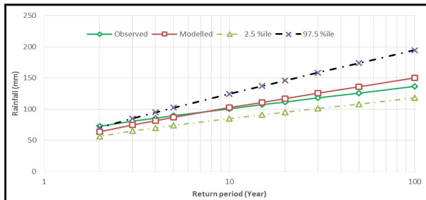
**Figure 11. Comparison of Gumbel estimated magnitudes of rainfall for studied return periods using observed and simulated AM series**
