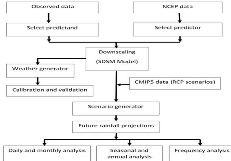
**Figure 2. Schematic illustration of the present study**
