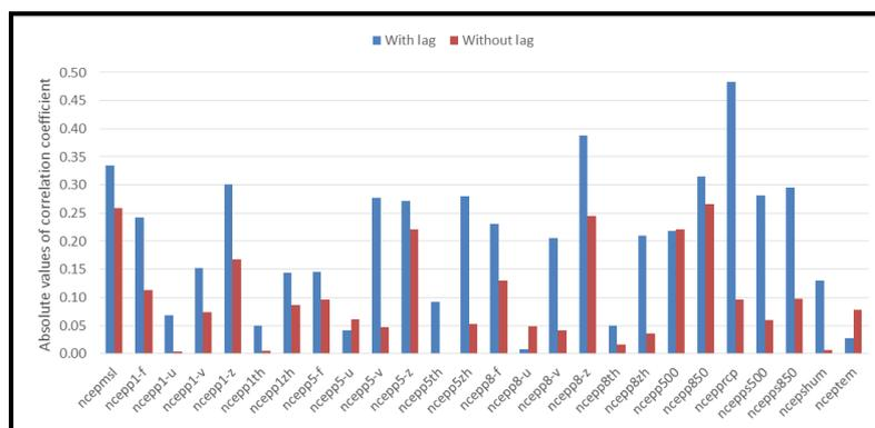
**Figure 3. Absolute values of correlation coefficient between the Lucas Creek rainfall and NCEP predictors with and without lag**
